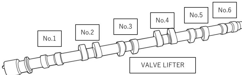
Be careful not to over tighten the cam cap bolts on lobes #1, #2, #4 and #6. Whilst these are easier to tighten than lobes #3 and #5, doing so will result in uneven vertical force, causing the camshaft to warp or even break.
